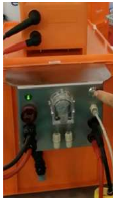
Figure 8: Magic box (Autofeed system)
