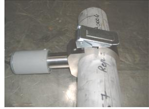
**Removing a hot spot from a pipe DN40 of 10 mSv/h on contact** (EDF).
